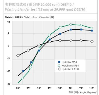
\* Waring Blender Test: A method to simulate the degradation resistance of effect pigment lacquers. The test, originally developed by an US located OEM manufacturer, allows comparisons of degradation resistance trends within short testing periods.
